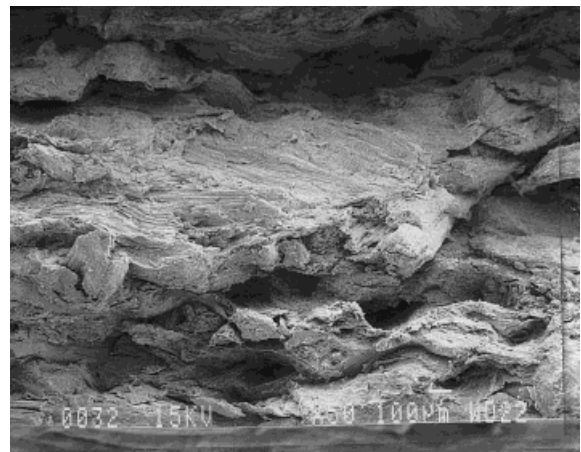
Figure 12 SEM of an esterified bagasse composite pressed at 190°C for 8 min. Ester content 42.5%.
